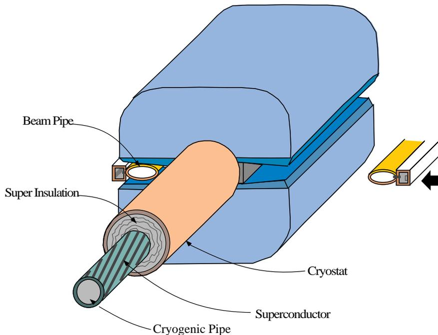
Fig. 1: Double-C twin bore transmission line magnet
