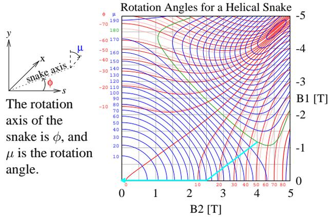
Figure 3: Contours of spin rotation for various values of the magnetic fields. Note that the  $\phi$  contours shift slightly from injection (red) at 25 GeV to storage (pink-light) at 250 GeV.
