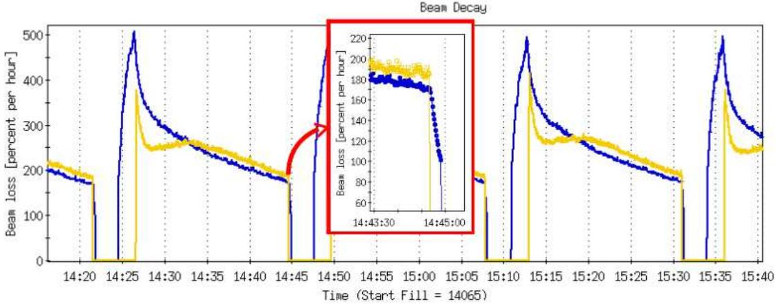
Figure 7: Beam decay rates during several  $\sqrt{s_{NN}} = 11.5$  GeV stores. At the end of each store, the Blue beam decay dramatically improves as soon as the Yellow beam is dumped (see insert). Note that the algorithm to calculate the beam decay has a time constant of 20 seconds. Hence, the actual drop in instantaneous beam decay is even more dramatic than suggested by this picture.
