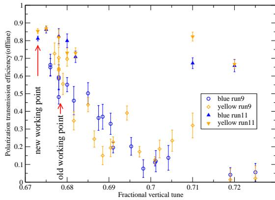
Figure 1: The polarization transmission efficiency on the energy ramp as a function of  $\nu_y$ . The open points are from run9 and the solid ones are from run11. The efficiency is improved in run11 and is about 85% at the new working point.
