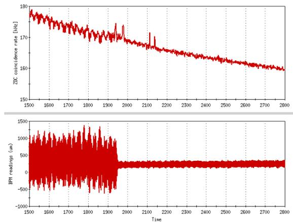
Figure 4: Collision rate with and without 10Hz orbit feedback as a function of time. Top: collision rate. Bottom: BPM signals with feedback off (<1950) and on (>1950).
