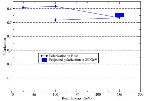
Figure 2: The polarization at various energies in RHIC blue ring. The projected 250GeV polarization is also shown as a band indicating error bars.
