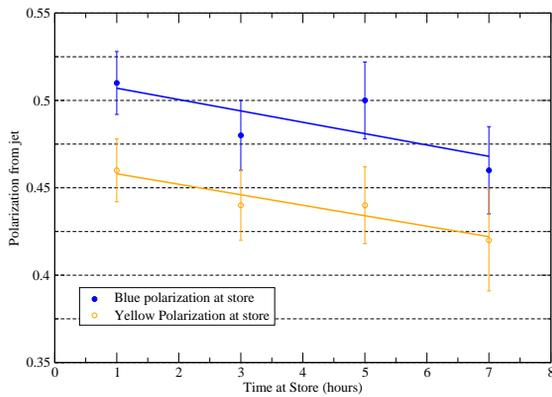
Figure 3: The polarization measured by the jet averaged over several long stores in both rings as a function of time.
