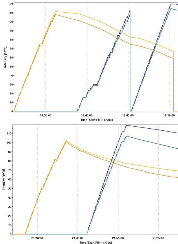
Figure 2: Beam intensities in the Yellow ring during injection of the Blue beam, at the FY2010 working point of  $(Q_x, Q_y) = (.13, .12)$  (top) and the FY2014 near-integer working point  $(Q_x, Q_y) = (.095, .085)$  (bottom).
