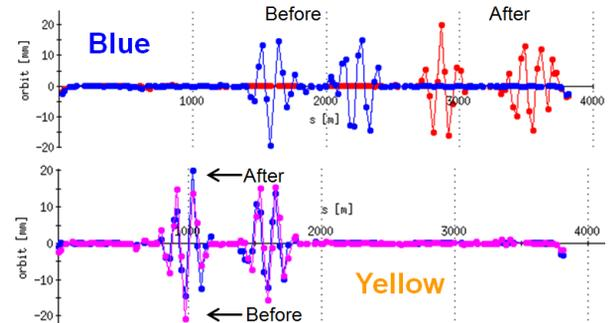
Figure 3: Closed orbit before and after protection bumps change.
