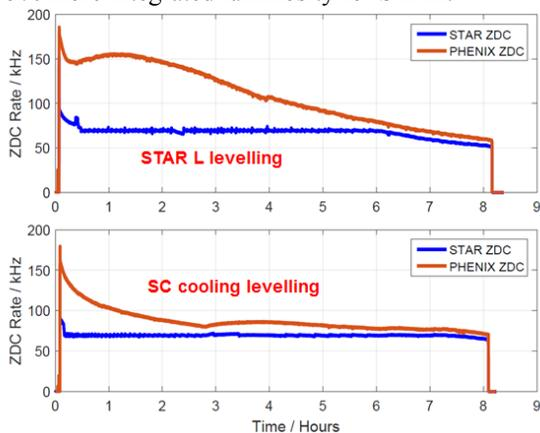
Figure 4: STAR luminosity levelling with 70 kHz ZDC rate (top); SC cooling levelling was used for higher integrated luminosity for STAR.
