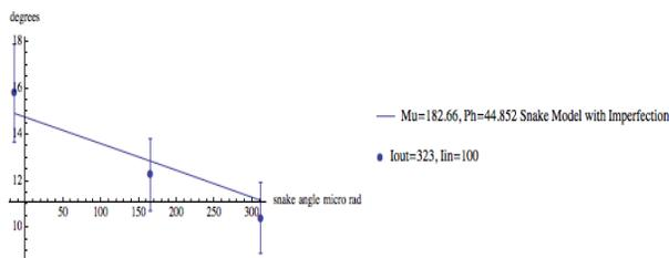
Figure 6: Response of average spin tilt at store in Blue ring to changes in the orbital angle between snakes. We compared response to simple model with snakes at settings based on model value for  $I_{in}=100$  and  $I_{out}=323$  amps with a strong imperfection source at  $G\gamma = 487$  (0.25).
