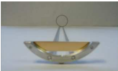
Figure 1: Picture of the STAR gold fixed target. The target was inserted in the lower part of the 75 mm beam pipe.
