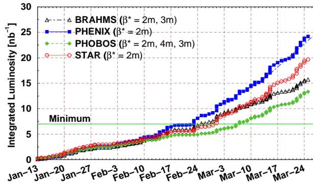
Figure 4: dAu run integrated luminosity. PHENIX integrated luminosity averaged  $4.6 \text{ nb}^{-1}/\text{week}$  near run end.
