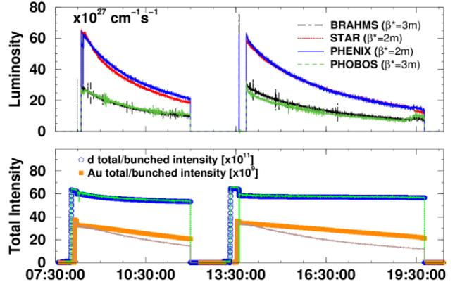
Figure 2: Two typical RHIC FY03 dAu stores, showing beam current ( $\times 10^{9/11}$  Au/p, total and bunched) and luminosity lifetime. Luminosity lifetime was dominated by gold beam lifetime and IBS-driven debunching and emittance growth. Time between stores was about 1 hour.
