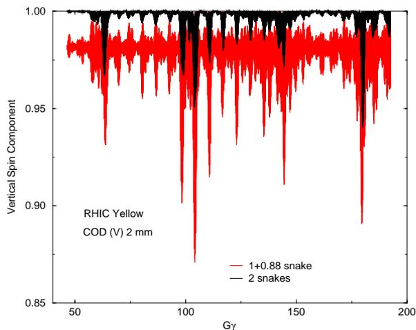
Figure 5: A single particle spin tracking for Yellow ring with two snakes and 1.88 snake scenarios. For the 1.88 snake case, the stable spin direction is not vertical.
