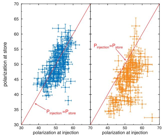
FIG. 1 (color). Achieved beam polarization at RHIC store (100.2 GeV) as a function of the beam polarization measured at injection (24.3 GeV) during the RHIC polarized proton 2005 run. The left plot shows the beam polarization in the Blue ring and the right plot is the achieved beam polarization in the Yellow ring.
