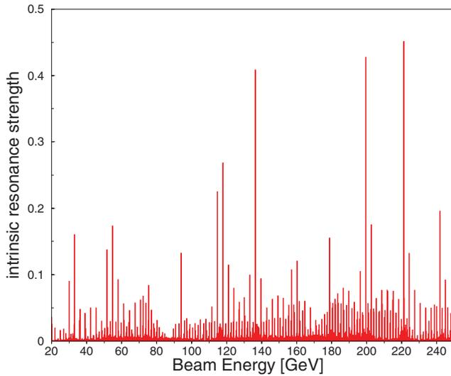
FIG. 2 (color). RHIC intrinsic spin resonance strength as a function of beam energy. This is calculated with a 2 m  $\beta^*$  at STAR and PHENIX, 3 m  $\beta^*$  at Brahms, 10 m  $\beta^*$  at PHOBOS, and 5 m  $\beta^*$  at the RHIC absolute polarimeter [18].
