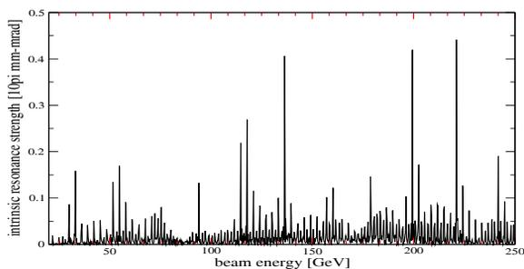
Figure 1: RHIC intrinsic spin resonance strength as a function of beam energy. This is calculated with a 0.7 m  $\beta^*$  at STAR and PHENIX, and 7.5 m  $\beta^*$  at all the other interaction points.
