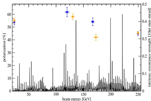
Figure 4: The solid blue circles and yellow diamonds are the measured polarizations of beam in the RHIC Blue ring and Yellow ring. The polarization measurements as function of beam energy are laid on top of the RHIC intrinsic depolarizing resonance strength as shown in Fig. 1 to guide eyes.
