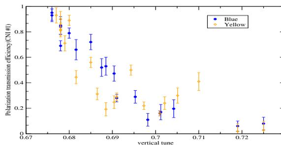
Figure 5: The polarization transmission efficiency in this plot is defined as the ratio of the polarization measured at store to the polarization measured at injection. For these measurements, only the vertical tune from 100 GeV up to 250 GeV was varied. The vertical tune below 100 GeV was kept around 0.68.
