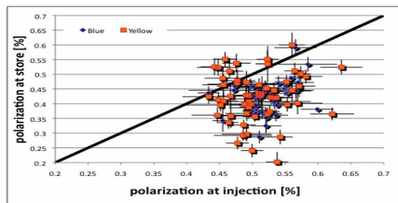
Figure 3: The plot is the polarization measured at store versus the polarization measured at injection using CNI polarimeter #1. Blue and Yellow are the two accelerators of RHIC. All the polarization measurements were done with profile-by-sweep mode, sweeping the target across the beam.
